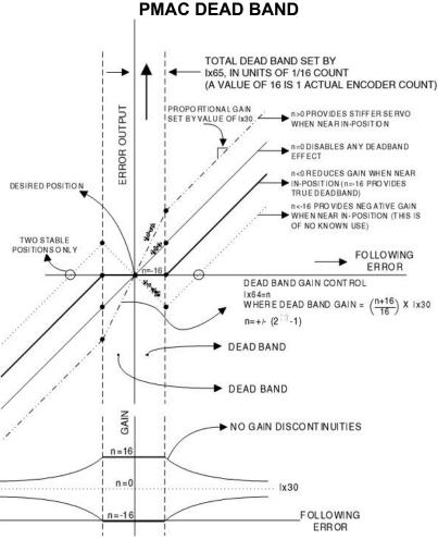
Values of Ix64 greater than 0 yield increased gain within the deadband; a value of 16 provides double gain in the "deadband". A small band of increased gain can be used to reduce errors while holding position, without as much of a threat to make the system unstable. It is also useful in compensating for physical deadband in the system.
